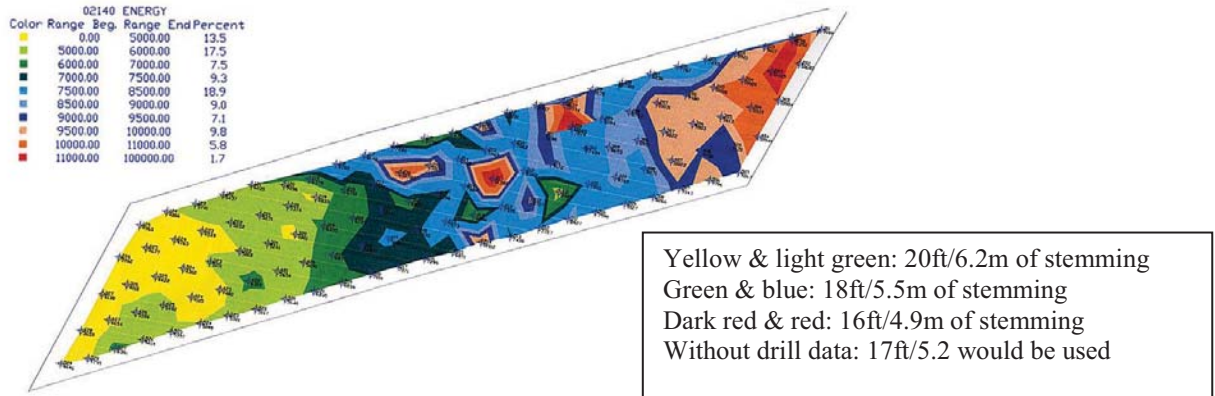
Figure 9: Drill pattern with calculated Specific Energy
